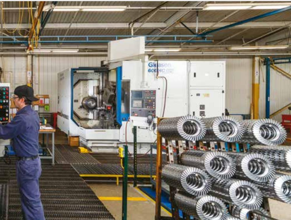
shown here operating the new Gleason 600HC, and one of three 600HCs that do all the spiral bevel gear
