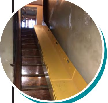
Purchased two 10' slide sections for use on large projects where material can be slid down the stairs. This helps mitigate risk of back and slip/trip hazards.
