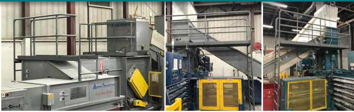
Platforms were added to the 125 HP baler area to provide for safe servicing of equipment. Bollards were also added to help prevent injury if pins fail on the balers.
