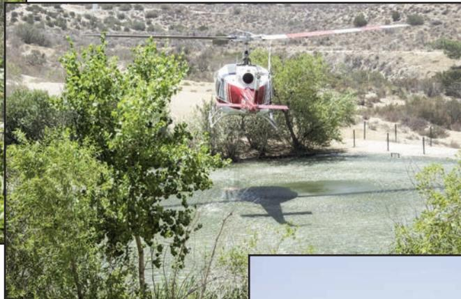
Here is a "Bambi bucket" lowering into the front edge of our pond away from our ducks. The chopper lets it sink into the water sending the fish away from it. Then with tremendous force the chopper lifts it out again and delivers it to the fire, knocking out the flames burning our forest, our wildlife, and their habitat.
