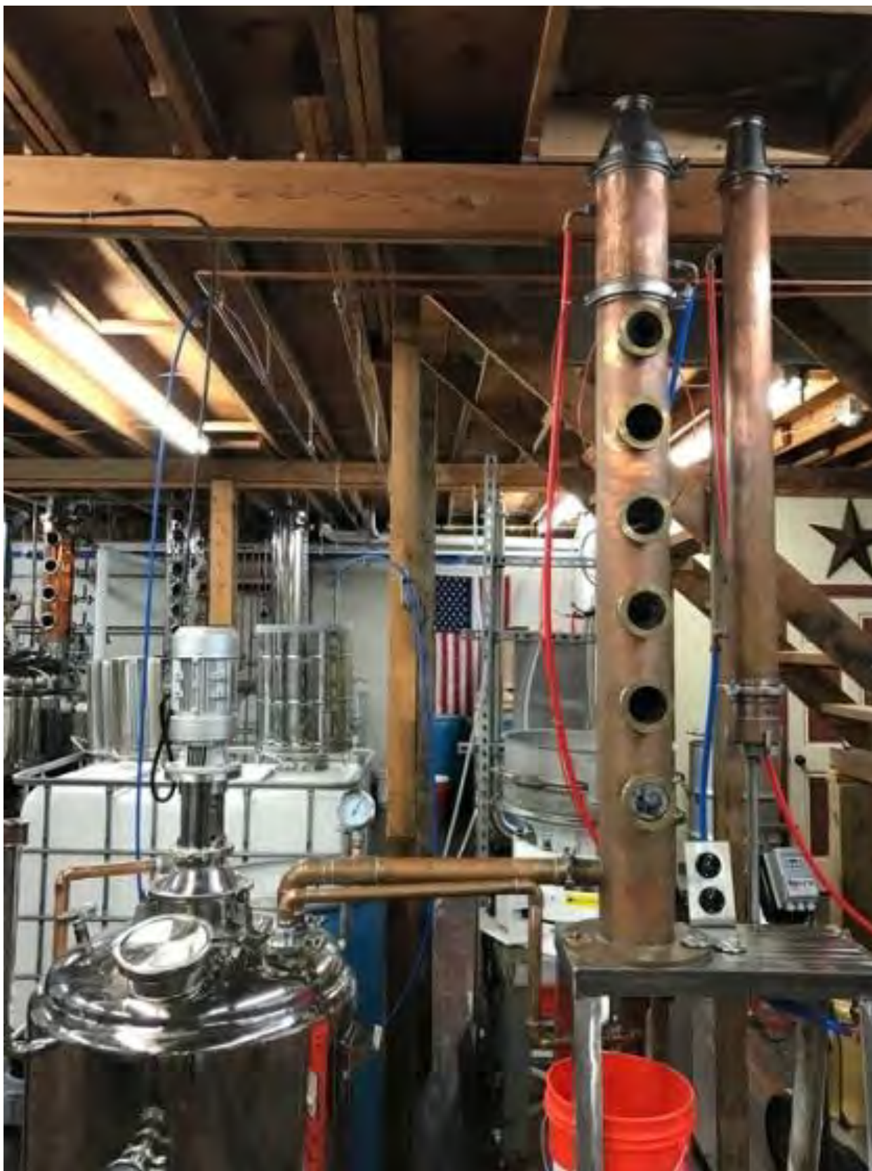
Homemade 6" column on original still
