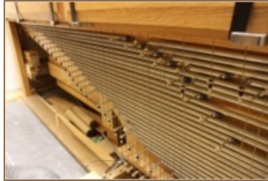
Slider chest: when stops are pulled, these levers shift to allow air to flow into a rank of pipes
