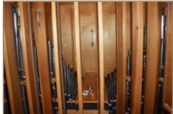
View looking in to the swell box-- these shades are controlled by the organist's foot on a pedal at the console
