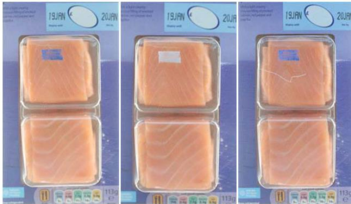
Photographs of oxygen indicator ink printed on a MAPed food package. Left: Before UV activation. Middle: After UV activation. Right: On opening the package. (Photographs: David Hazafy, University of Strathclyde)
