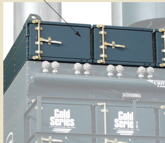
Below: Dust collector with integrated HEPA safety monitoring filter
