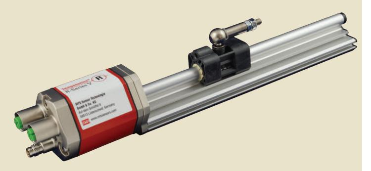
To replace the sensor, the sensor cartridge is unthreaded, the sensor electronics are replaced, and the sensor cartridge is reinstalled into the cylinder. MTS developed this method to allow for easy exchange of the sensor cartridge while the pressure seal is maintained, avoiding possible oil spillage and contamination.
